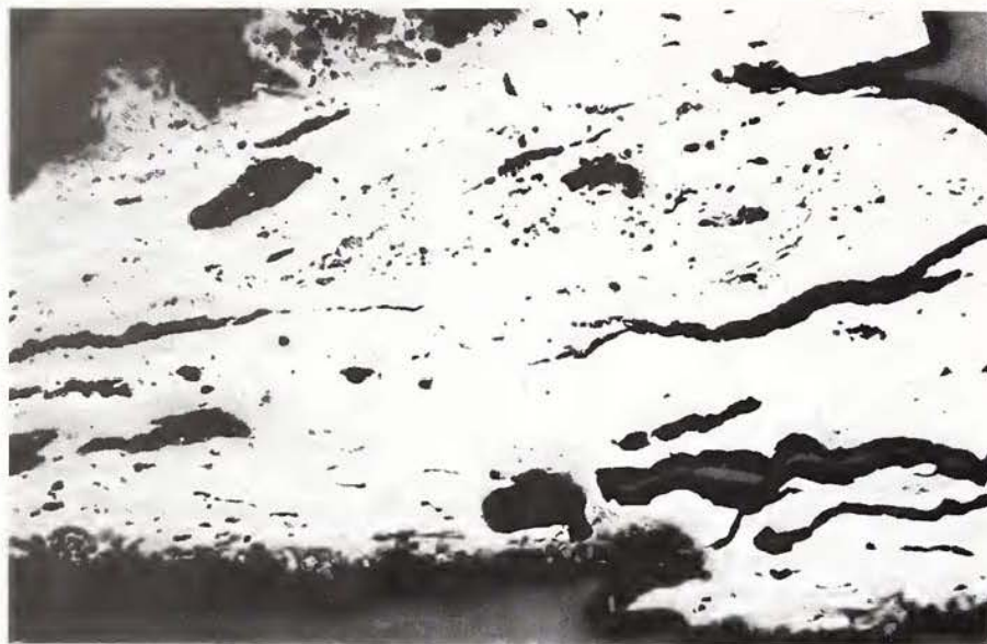
Fig. 13. Polished transverse section through corroded spatula, Cong 21, showing disruption of the structure through heavy corrosion (28 X).
