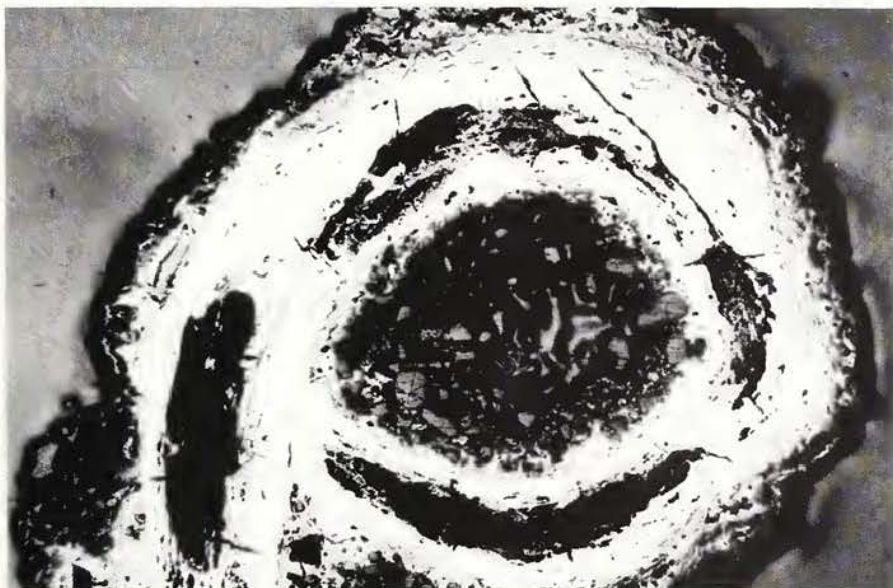
Fig. 11. Polished longitudinal section through the eye of pendant, Cong 10, showing neatly forged abutment of folded over end against the shaft (14 X).
