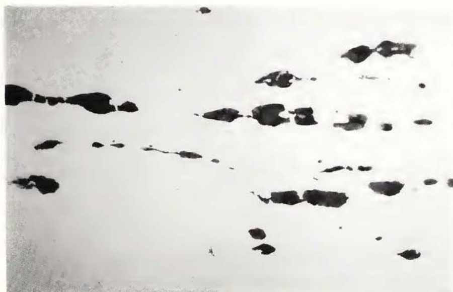
Fig. 5. Polished longitudinal section through iron bar, Cong 5, from Loubanzi, showing typical elongated two-phase bloomery iron inclusions consisting of wüstite droplets in dark glass (360 X).
