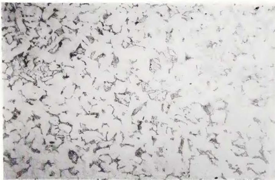
Fig. 8. Longitudinal section through iron bar, Cong 5, from Loubanzi, etched in nital, showing area of approximately 0,1 % carbon composition (450 X).
