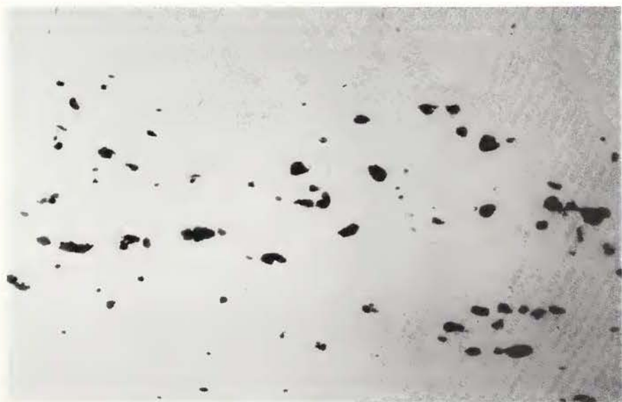
Fig. 6. Polished longitudinal section through iron bar, Cong 5, from Loubanzi, showing fractured and rounded two-phase inclusions indicative of heavy hot working (225 X).
